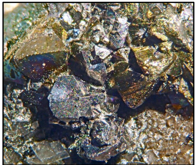
Siegenite (silvery) and Chalcopyrite (gold). Sweet-Water Mine, Reynolds County, MO. FOV 5 mm. Photo by Michael Pabst, using stereomicroscope, stacking 13 images.
