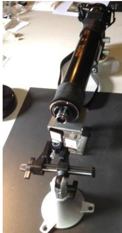
Figure 3: Assembly for photomicrography, including (from front to back) the sample stand, micrometer stage, micromount box, 40 mm Luminar lens, velvet-lined tube, bellows, and Panasonic mirrorless camera.
