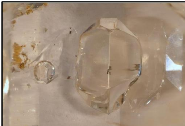
Figure 1 Negative quartz crystal (4 mm top to bottom). Note the irregular void to the left with a round object. The sphere does not move and seems to have some flat faces.
