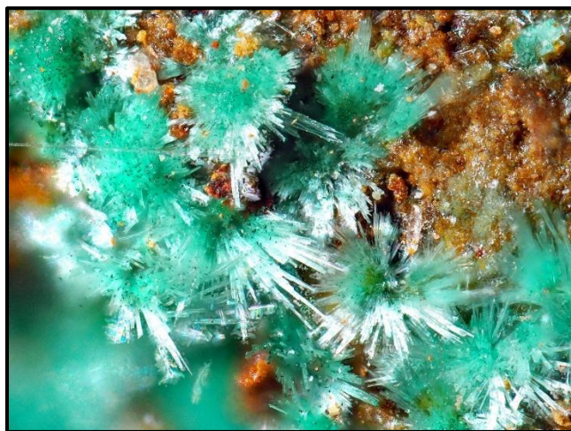
Pauladamsite. Santa Rosa Mine, Inyo County, California. FOV 1 mm. Photo and specimen by Michael Pabst, using WeMacro computer-controlled rail ($400) with Mitutoyo M Plan Apo 10X infinity-focus lens ($1000), stacking 24 images. Illumination by indirect daylight.
