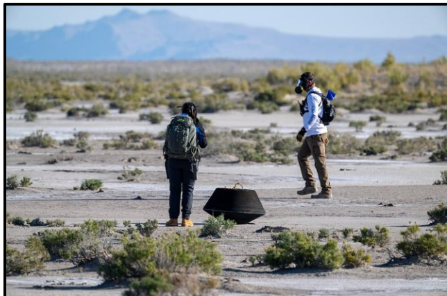
Fig. 5: OSIRIS-REx sample return capsule just after landing in Utah on Sept 24, 2023, with members of the recovery team. Credit: NASA/Keegan Barber via Wikipedia.
